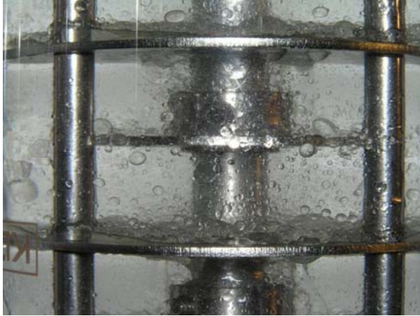
Figure 5.5. Photo of column contents when the organic phase is continuous and the ionic liquid phase dispersed, T = 75\text{ }^{\circ}\text{C} , F = 10.8\text{ m}^3/\text{m}^2.\text{hr} and N = 643\text{ rpm} .
